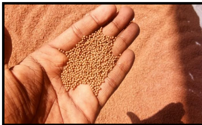
Figure 6: Grinding media (Zirconium Beads) [Dt.07-09-2018, Time -03:05:00]
