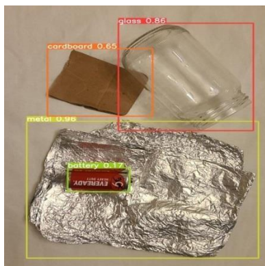
Fig.4.2. YOLOv6 waste detection results
