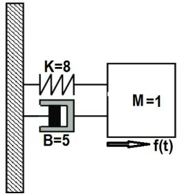
Here the system can be modeled by solving the differential equation of the system using the application of Laplace Transform. Herein, M(Mass of block) = 1, K(Stiffness of Spring) = 8 and B (Damper) = 5.
