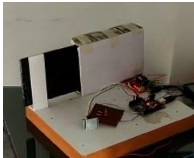
Figure 5: Automatic open door system model
