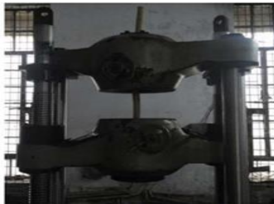
Figure 7: Tensile Strength Test of Bamboo stick
