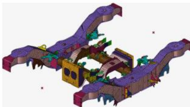
Fig. 4. Finite element model of Bogie Frame
