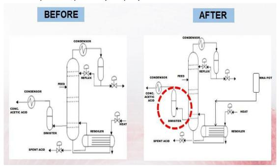
With the effective maintenance of distillation column we were finally achieved the aimed target of decolourizing of acetic acid, increase in the rate of production with minimum inputs and high quality. Following rate of production we got as far:-
