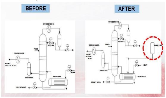
As thoroughly undergo study we found that we need to install intermediate WNA pot which acts as an intermediate anti rusting agent and to increase the height of heating column along with installation of demister
