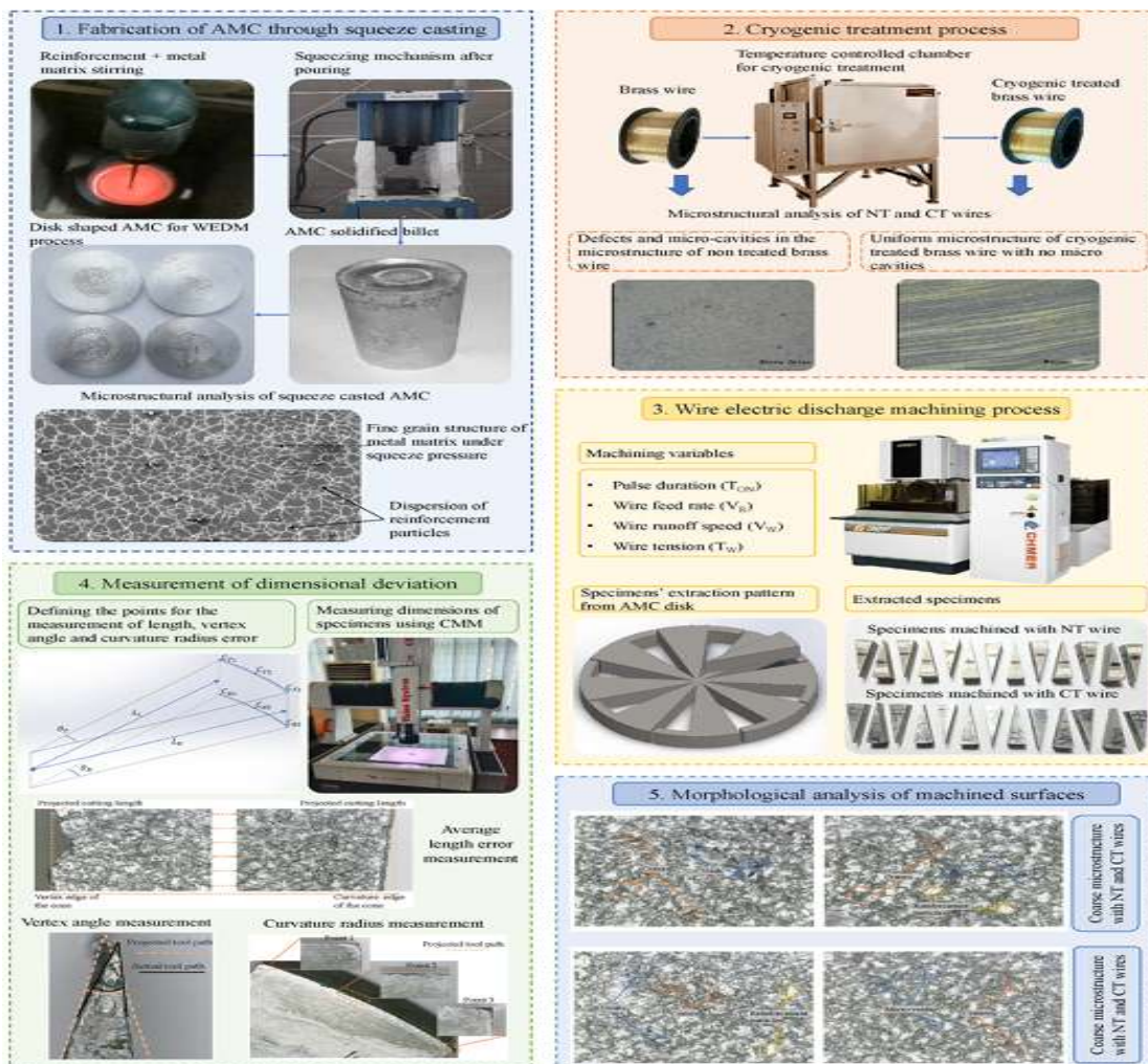
Figure 4: Experimental procedure and Microstructure Analysis of Machined Surfaces [10]
