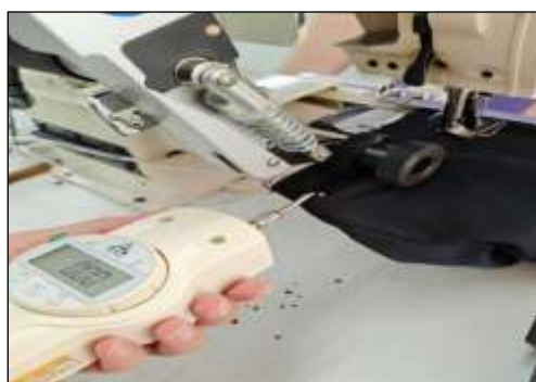
Figure 9: The measurement of the pulling experiment at the beginning stage
