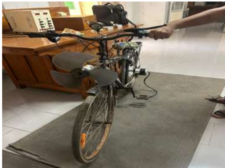
Fig 6: Integration of wind Harvesting System to Electric Cycle
