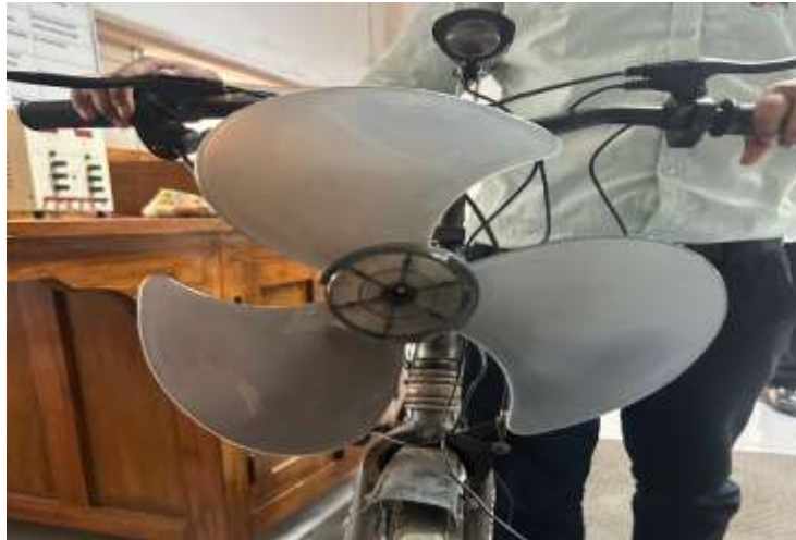
Fig 5: Wind Harvesting System
