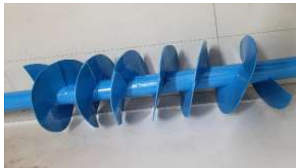
Figure 3: PVC Turbine Design
