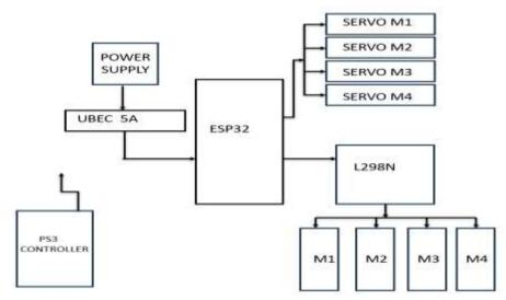
Commands are transmitted from the PS3 controller to the ESP32, which interprets them and produces the proper control signals for the L298N motor driver. The four motors are then driven by the L298N, which moves the robotic arm in the appropriate direction and at the required speed.
