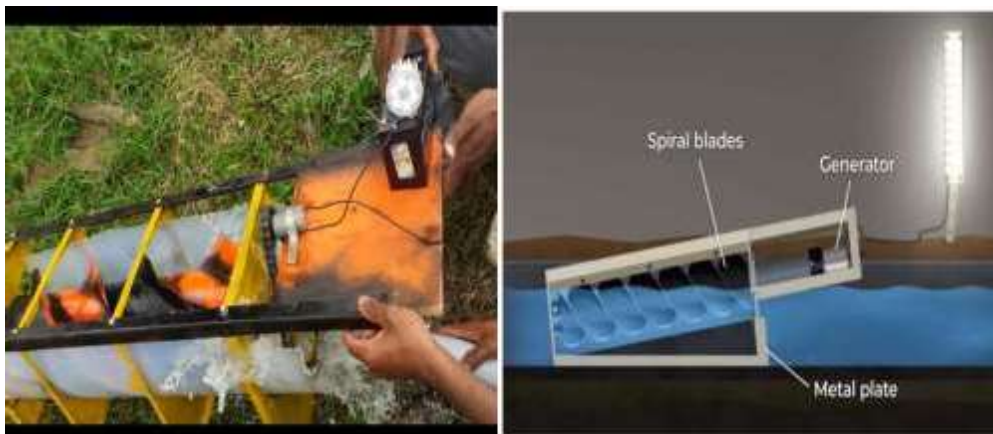
Figure 4: Overall view of Pico hydro power generation using spiral turbine
