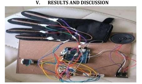
The results from functional testing indicated that the system successfully identified gestures with an accuracy rate of over 95%. The audio feedback provided clear, audible responses, and the OLED display delivered real-time updates without significant delays. Usability trials with end-users revealed that the system was intuitive to operate, with minimal physical effort required to perform gestures.
