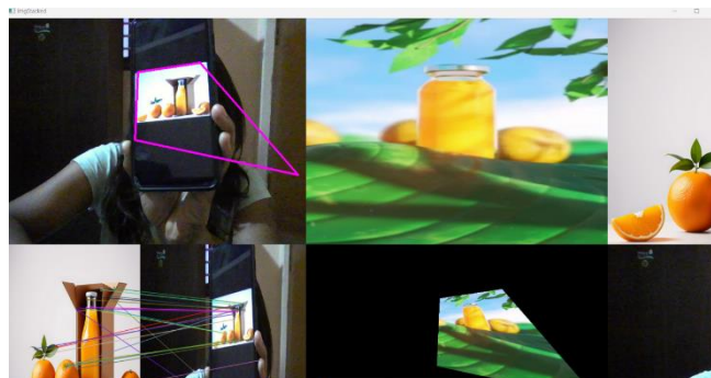
Figure 3: Initializes a Brute Force matcher to compare keypoints between the target image and the webcam feed.
