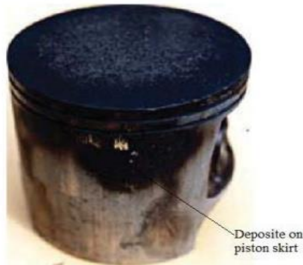
Figure 4. Piston skirt shows deposition [2]
