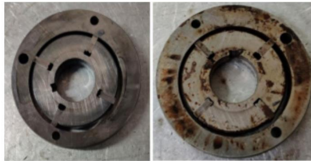
Figure 19. Original and failed veins of supply pump [19]
