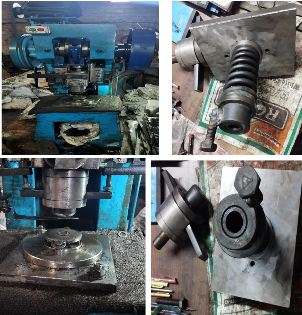
Fig 18: Actual pictures of mechanical power press , die plate, die block and spring holding Pipe
