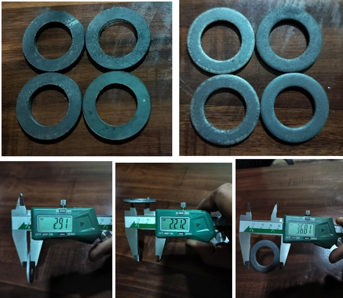
Fig 20: Manufactured product ( M20 plain washer) and dimension under IS2016 standard
