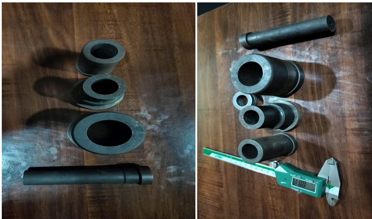
Fig 19: Actual Pictures of Piercing punch, Blanking die, Lower die and Injector
