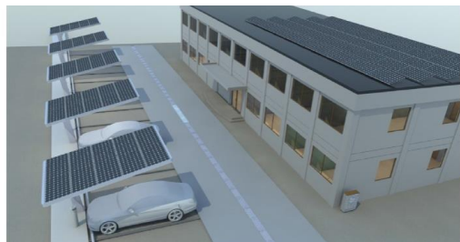
Figure 2: Design of solar powered EV charging station.
