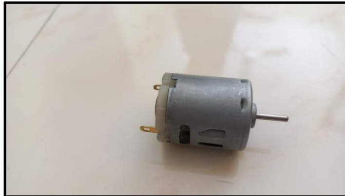
Figure 10: DC Motor (Side View)
