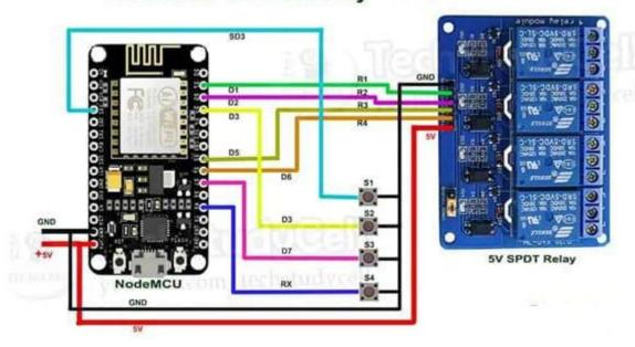
The circuit for this Node MCU home automation project is very simple. Here I have used an active low 5V relay module. I have used the **INPUT\_PULLUP** function in the code instead of connecting pull-up resistors with the push buttons.
