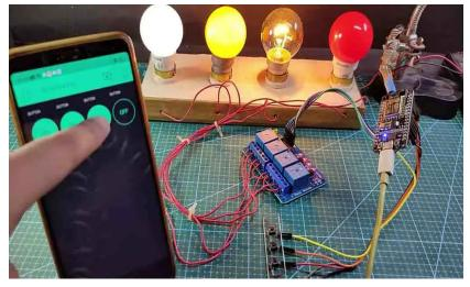
Now, you can easily control the home appliances from the smartphone using ESP8266 wifi module. And you can also monitor the real-time status of switches in the android software.
