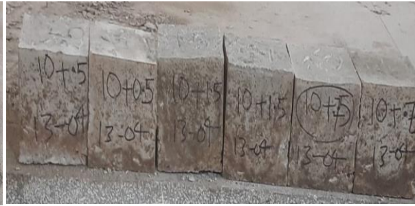
Fig 4: Specimen of Beams
