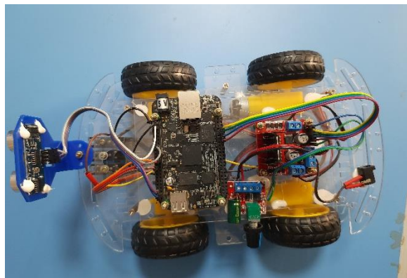
Fig. 4. Autonomous Car using BeagleBone Black
