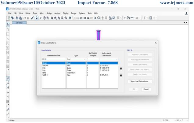
According to the specifications outlined in EN 1990 and EN 1998-1 the design of the stack should take into account the following load factors:
