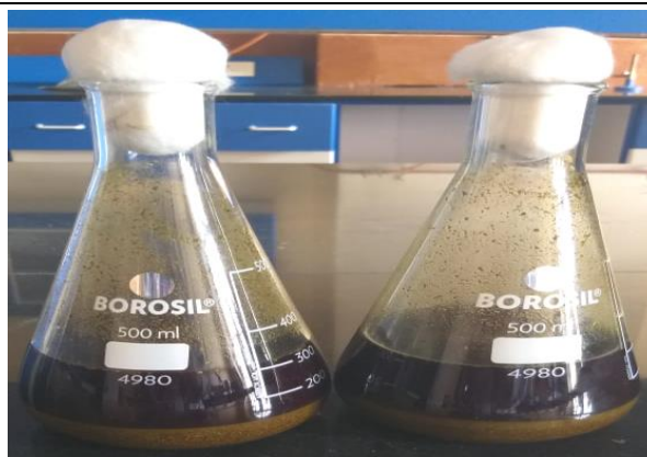
Fig 3.4.1: The powdered sample of C.sinensis soaked in ethanol solvent for crude extraction
