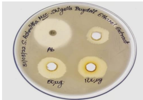
Fig 3.6.5: The zone of inhibition of test sample against S.buydoii ; Ab- Gentamicin as standard
