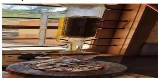
Fig 3.4.2: The aqueous extraction of C.sinensis in Soxhlet apparatus
