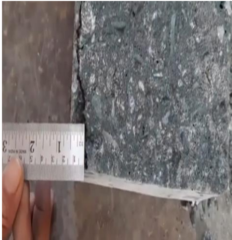
Fig:9 water permeability test at 28 days
