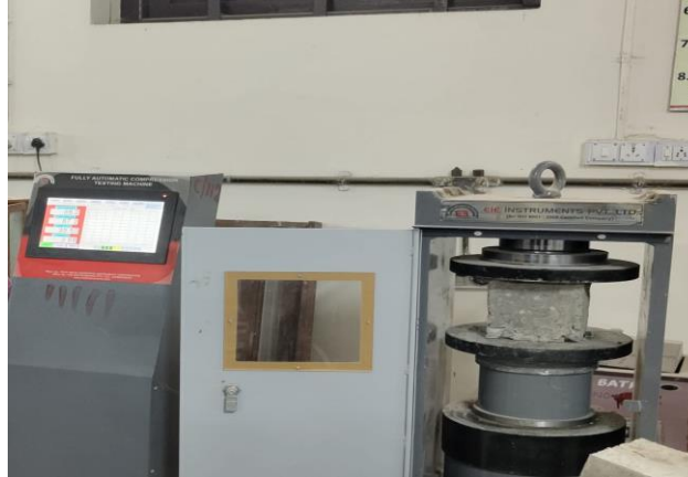
Figure 4: Compressive strength testing
