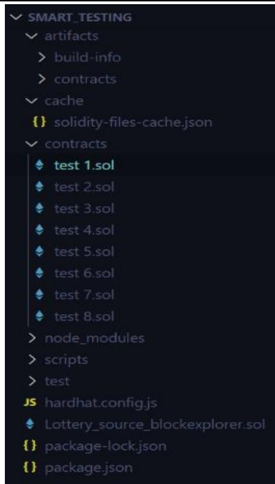
Figure 3: File management in VS Code after hardhat installation.
