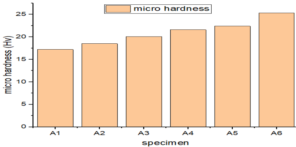
Fig. 3: Variation of Hardness value w.r.t to nano-Al 2 O 3 Content in composites.
