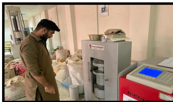
Figure 3: Compressive Test of Concrete Cube
