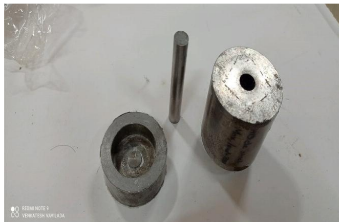
Figure 6: Punch and Mould used for compaction
