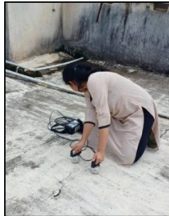
Fig. 3: Ultrasonic pulse velocity test
