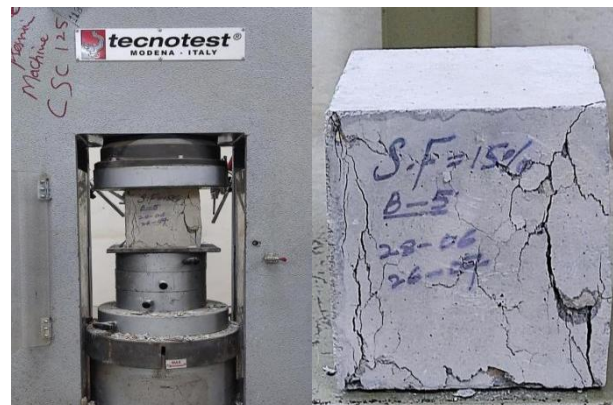
Figure 6: Cubes specimen under testing
