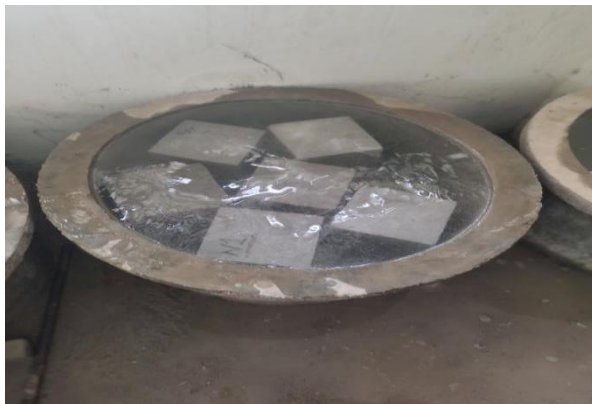
Figure 5: Curing of specimens for 28 days
