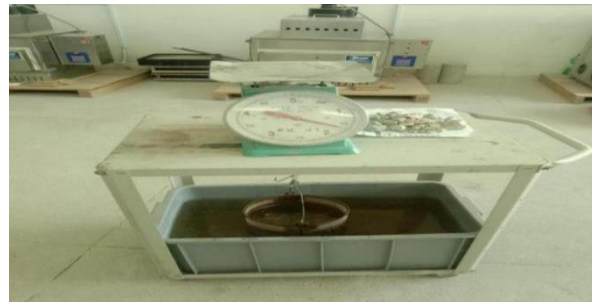
Figure 4: Water absorption and specific gravity test
