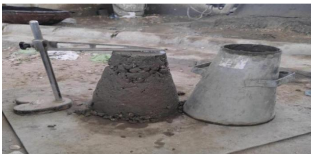
Figure 3: Pictorial view of Slump cone test
