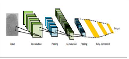
Figure 4. Architecture of convolutional neural networks. From [13].
