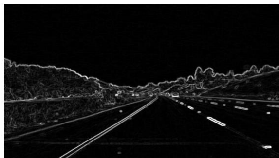
Figure 5: Canny Edge Detection
