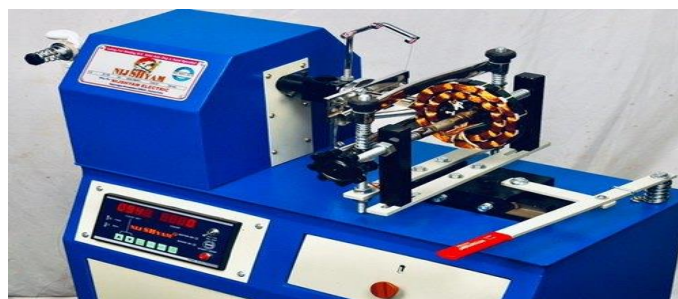
Fig 1: Automatic Coil Winding.
