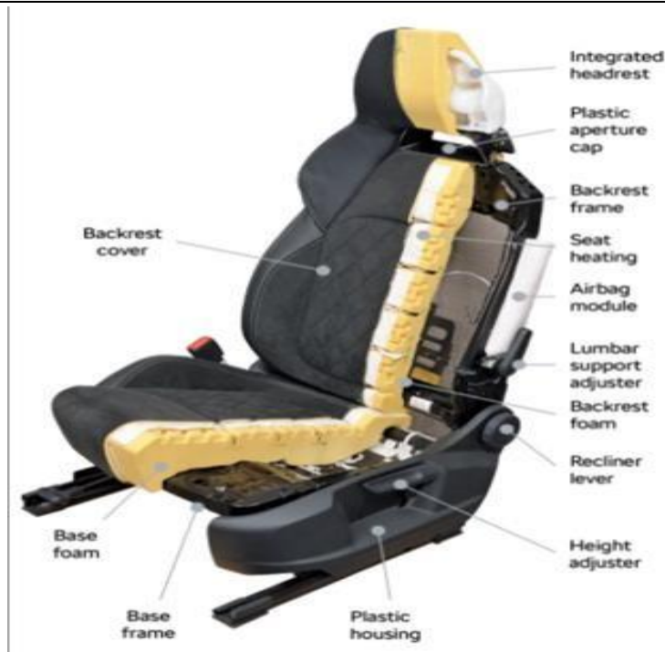
Figure 2: Cut-section of car seat and its components
