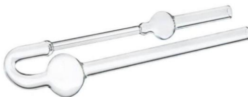
Fig.No.04. Ostwald's Viscometer
