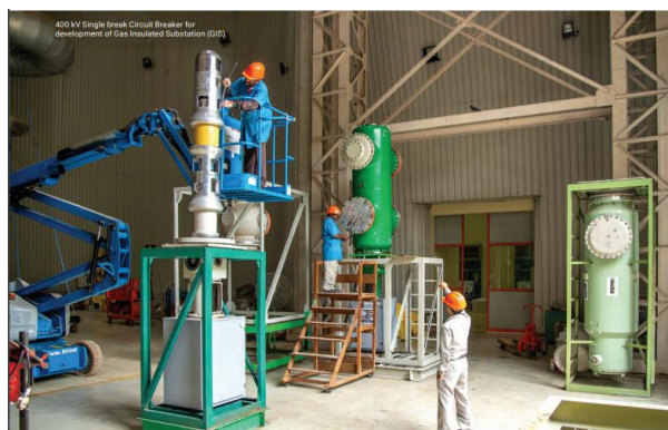
Fig.5 development of gas insulated substation (GIS)
