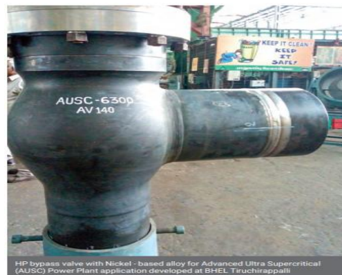
HP bypass valve with Nickel-based alloy for Advanced Ultra Supercritical (AUSC) Power Plant application developed at BHEL Tiruchirappalli
