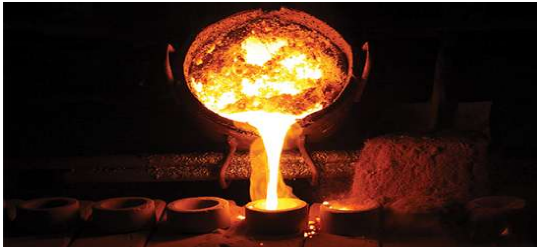
Fig-3: Pelting of molten metal into mould box .To get the required product through casting, then after 15 minutes of stirring, the liquid metal with reinforcement namely E-GLASS (0.120kg) and flyash (0.09kg) are pelting into the splitup types of dies to get the required shape of product through stir casting.(E-waste Al 6063 2 kg +copper 0.8kg+ E-glass fiber 0.12 kg + fly ash 0.15 kg).
