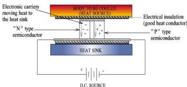
Figure:6 Working Principle of Peltier Module.
