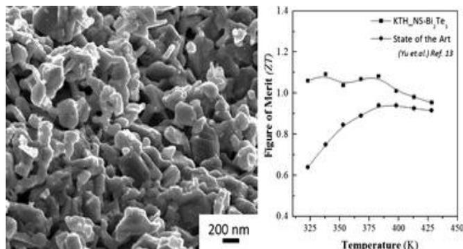
Figure:4 Microscopic Nano-Structure of Bismuth Telluride.
