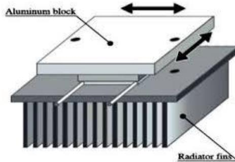
**Figure:7** Peltier Module on Aluminium block for better heat transfer.
