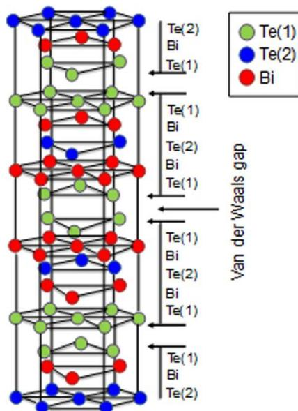
Figure:3 Hexagonal Nano-Structure of Bismuth Telluride.
