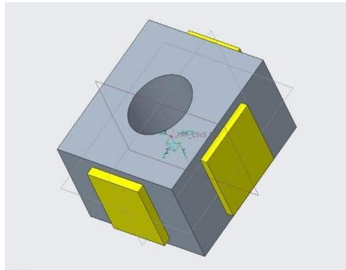
Figure:9 Peltier module (yellow) mounted on Aluminium block (grey)
