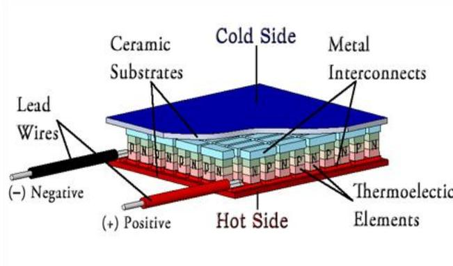
Figure:1 Construction of Peltier Module.
