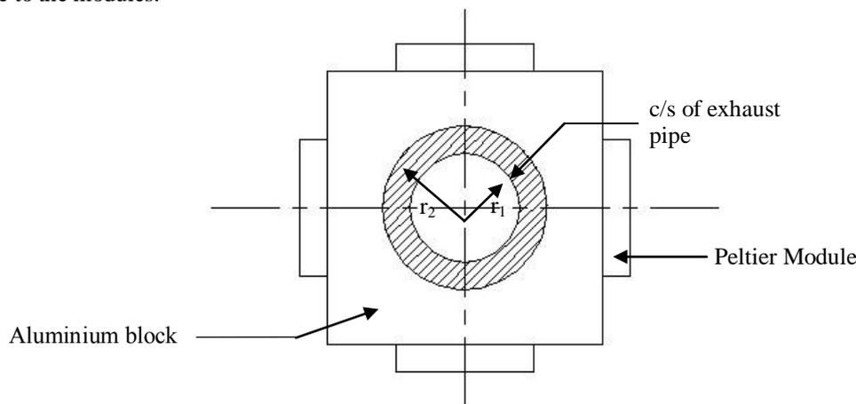
Figure:8 Heat transfer through aluminium block
