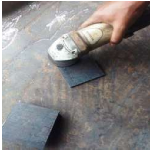
Fig. [3] Surface Cleaning.
