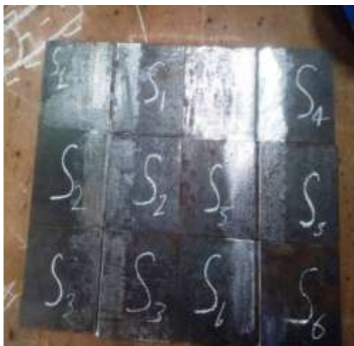
Fig. [5] Prepared sample for welding process
