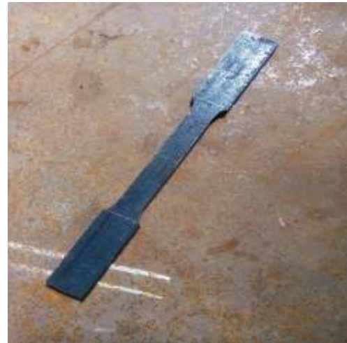
Fig. [6] Prepared tensile test specimen of base metal
