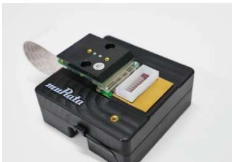
Fig-10: FET based biosensor instrument manufactured by matsumoto lab and muRata co. ltd.
