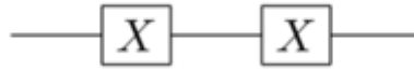
Fig-8: A multi X gate Quantum Circuit, comprising of two X gates in a row
