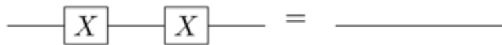
Fig-9: A multi X gate Quantum Circuit, comprising of two X gates in a row, as a Quantum Circuit is equivalent to a single quantum wire quantum circuit
