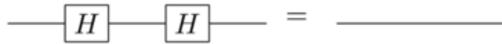
Fig-9: Net effect of the Quantum Circuit, as depicted in Figure 6 above, is the same as that of a Quantum Wire
