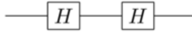
Fig-6: A simple Quantum Circuit that involves the use of two HADAMARD Gates
