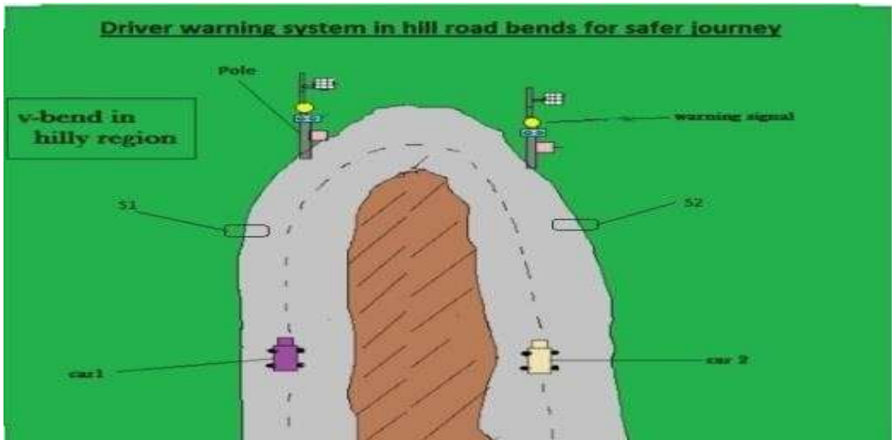
Fig-4: Driver Warning System
