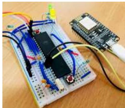
Fig-6: ATMEGA16 Microcontroller Testing
