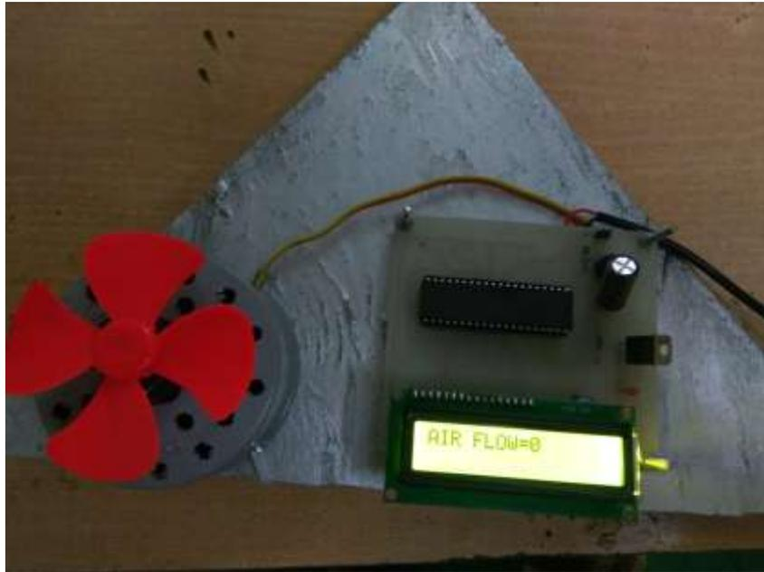
**Fig-12:** Flow Meter Designed For Asthma Detection
