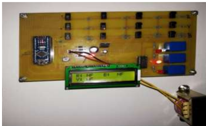
Figure-4: No fault condition
