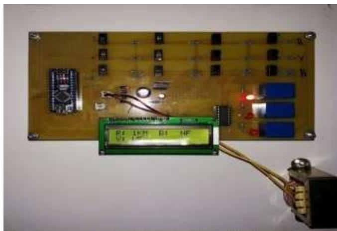
Figure-5: R phase short circuit condition
