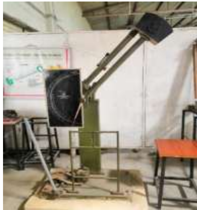
Fig-6: Impact Testing Machine & Tested Material
