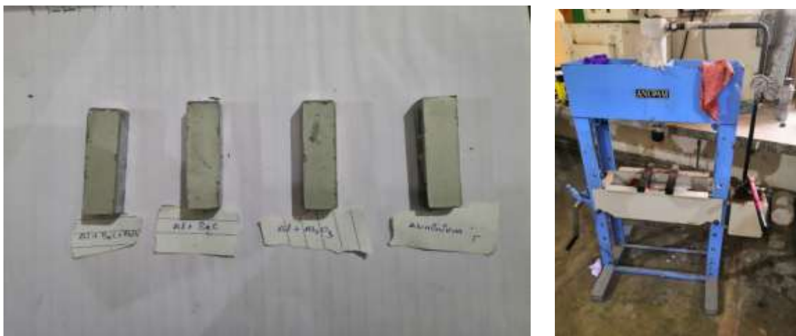
Fig-3: Compacted sample & Compacting Machine
