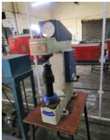
Fig-7: Rockwell Hardness Testing Machine & Tested Material
