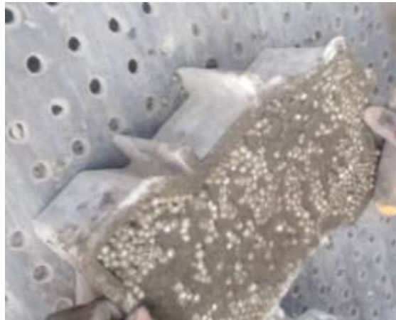
Fig-1: Paver Block with Polystyrene beads
