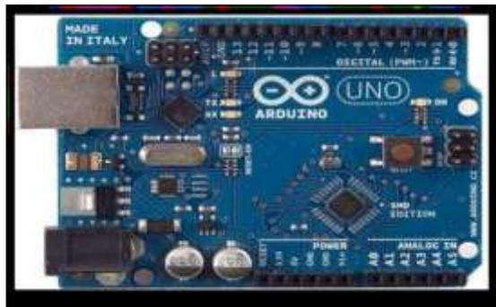
Fig-1: Arduino UNO board
