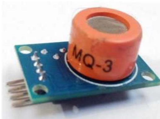
Fig-8: MQ3 Alcohol sensor
